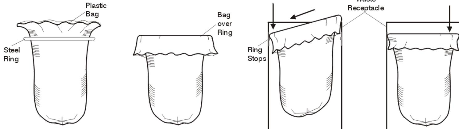
1. Bring the top of a new plastic trash bag up through the center of the steel ring.
