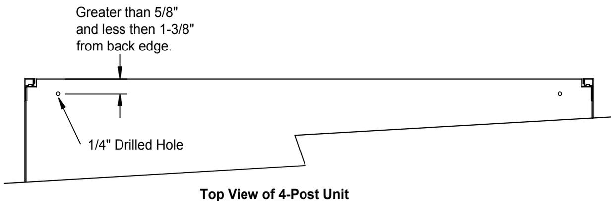
3. Drill a 1/4" diameter hole at the locations that were just marked on the 4-Post unit. Use a clamp to secure the shelf and shelf support together during drilling.
