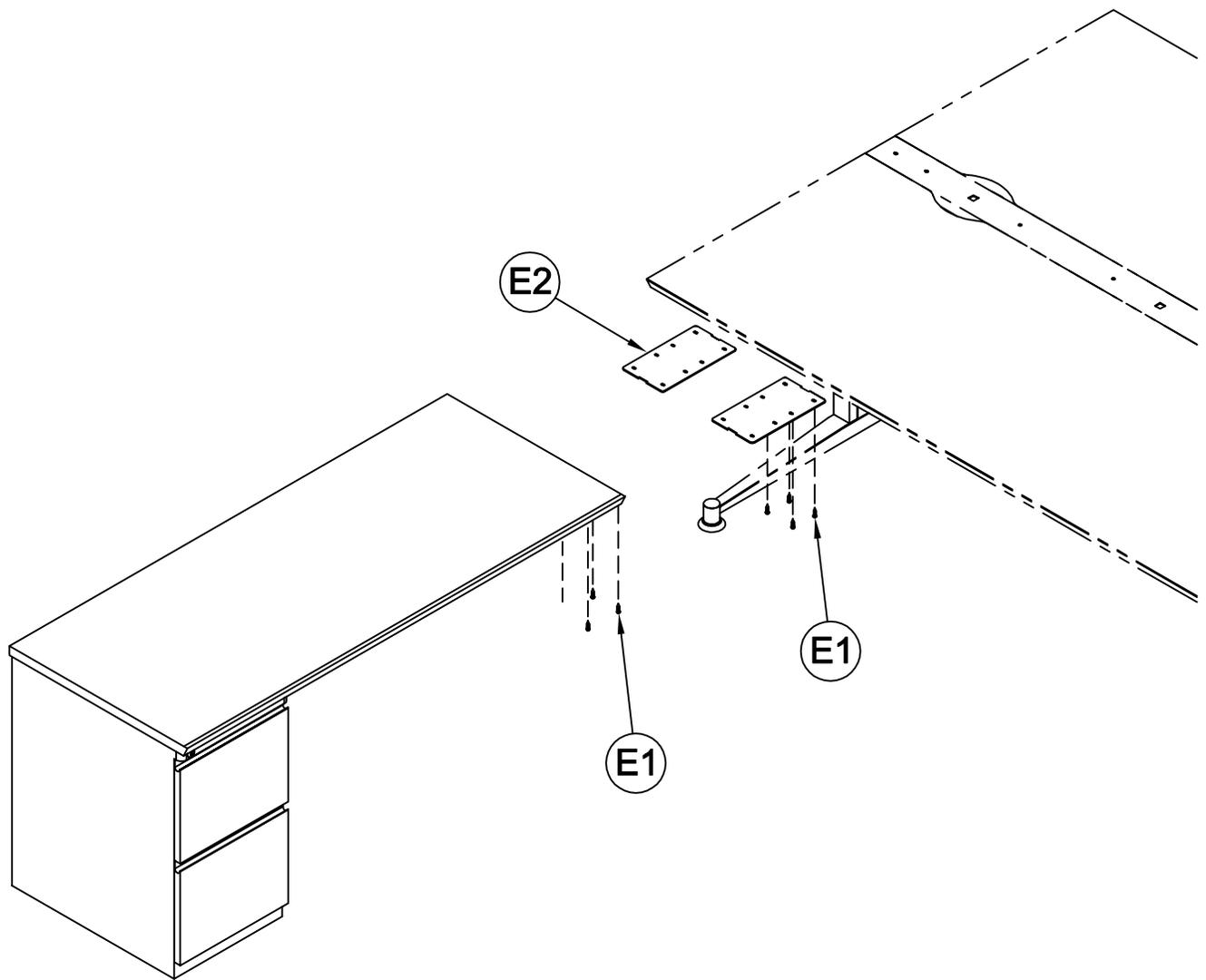
6. Align the holes in the two Joining Plates (E2) with the pre-drilled holes in the underside of the Adjacent table Work Surface. Attach each Joining Plate (E2) using four Screws (E1).
