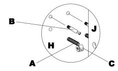
NOTE: The arrow on the face of the Cam (C) should point towards the Cam Post (B) for proper alignment.
