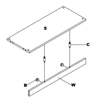
NOTE: The arrow on the face of the Cam (B) should point towards the Cam Post (C) for proper alignment.
