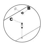
(2) Insert Wood Dowel (A) into Bottom (T). Install Cam Posts (C) into Back Panel (U). Insert Cam (B) into Bottom Panel (T). Attach assembled Bottom to Back Panel (U) by turning Cams (B).
