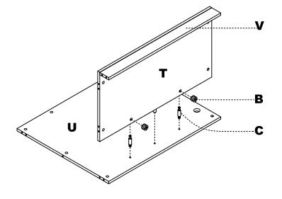
Insert Wood Dowels (A) into Back Panel (U), Bottom Panel (T), and Toe Kick (V). Install Cam Posts (C) into L.H. Side Panel (P) and R.H. Side Panel (Q). Insert Cams (B) into Back Panel (U), Bottom Panel (T), Toe Kick (V) and Cross Braces (R). Attach Side Panels (P & Q) and Cross Braces (R) by turning Cams (B).
